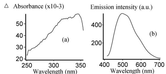
Fig. 2. (a) Differential absorbance spectrum between the irradiated and nonirradiated regions; (b) emission spectrum (excitation wavelength,  $365 \text{ nm}$ ) of the irradiated region. Experimental laser irradiation conditions:  $I = 6 \times 10^{12} \text{ W cm}^{-2}$ ,  $N = 10^6$ . Differential absorbance and emission spectra are assigned to laser induced  $\text{Ag}$  clusters.
