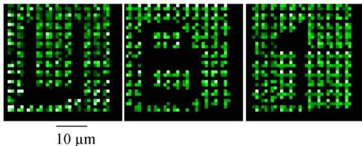
Fig. 3. (Color online) THG readout of the three layers containing the bit patterns U, B, and 1, recorded in the bulk of the glass (bit spacing, 3  $\mu\text{m}$ ; layer spacing, 10  $\mu\text{m}$ ). Laser writing parameters:  $I=6 \times 10^{12}$   $\text{W cm}^{-2}$ ,  $N=10^6$ . The three THG images present high signal-to-noise ratio and no cross talk.
