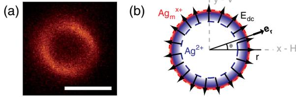
Fig. 1. (Color online) (a) Confocal fluorescence image of a photo-induced ring structure with an excitation at 405 nm. The scale bar is 5  $\mu\text{m}$ . (b) Schematic representation of a possible radial distribution of the silver species inside the ring. The permanent electric field is  $E_{dc}$ .
